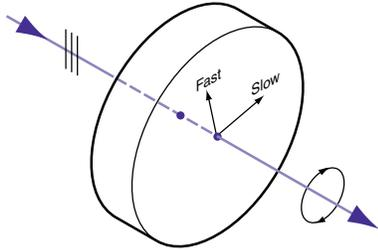
The construction of a Quarter Waveplate is such that the fast axis lies in the surface at 45° to the input polarization. The input beam is therefore resolved into two components of equal amplitude but varying velocities.
